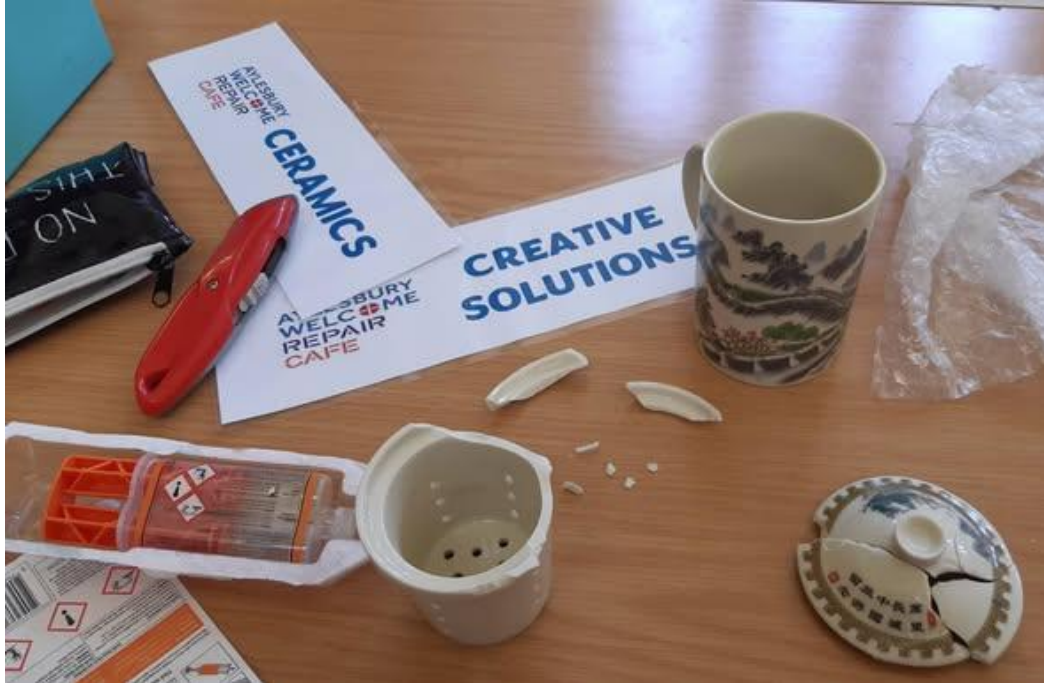
Ceramics can take more than one session to fix. Gluing or putty often needs a 24-hour curing phase. This Japanese patterned mug, infuser & lid will be coming back next session for further fixing and filling.
